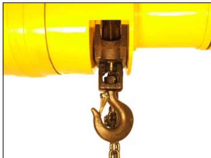
Figure 3-1c. Lower Block Contacting Stop Shoe at Upper Limit of Travel (electronic limit switch)
